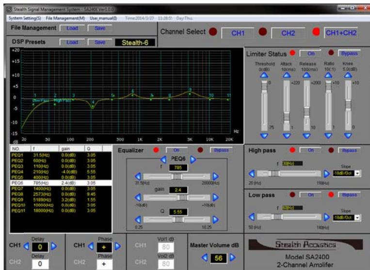
The SA2400's comes pre-optimized from the factory set to power the specific SPT speaker compliment. Utilizing Stealth's free SSMS software, the field installer can further adjust the SPT speaker tuning for best results.
